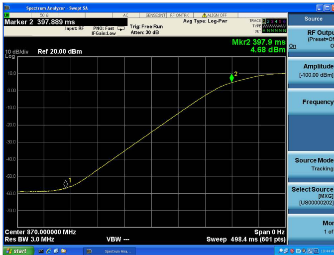
Figure 4. Power sweep mode shows gain compression, cut-off level, and linearity.
